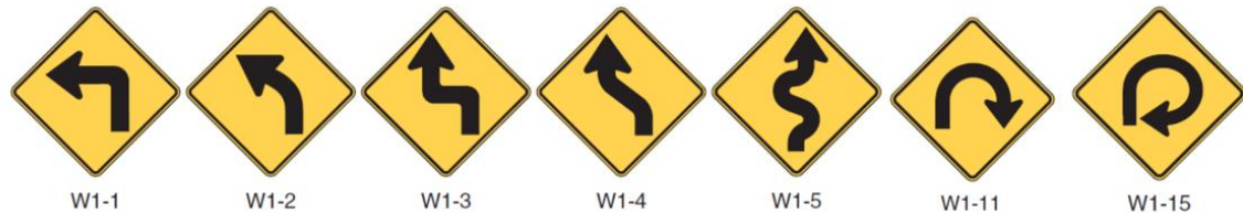
Figure 1.1 – Advance Curve Warning signs for horizontal curves.
