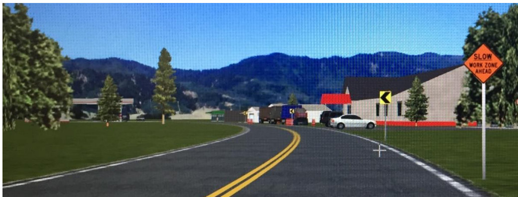
Figure 2.4 – SLOW: WORK ZONE AHEAD sign.
