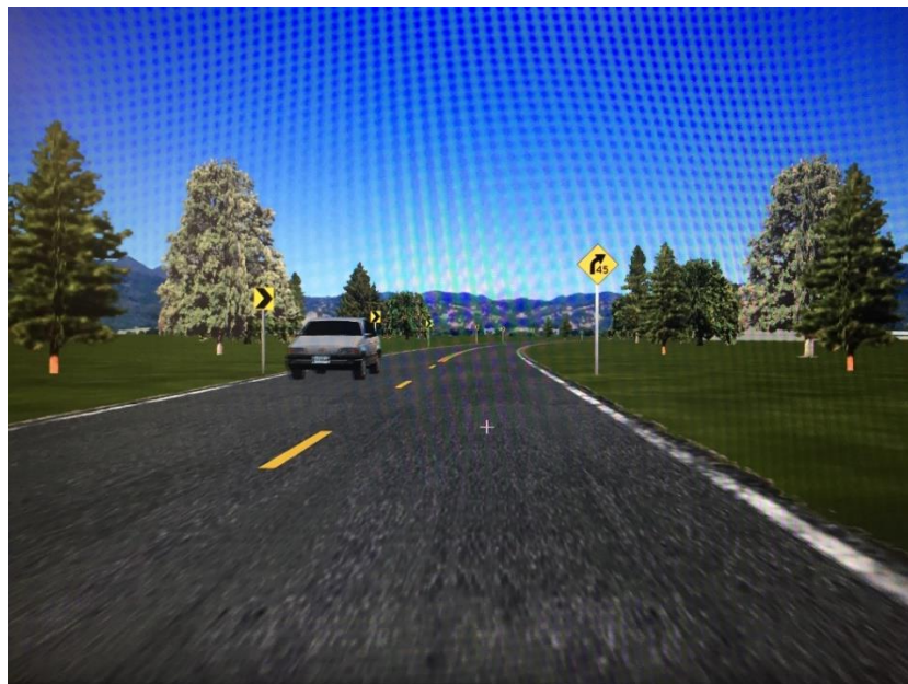
Figure 2.3 – Scenario showing Advance Curve Warning and Chevron signs.
